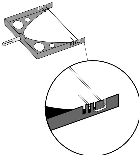
When mounted on the End Stops, these bumpers may also be used as glider launchers:
