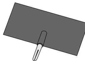
The glider itself may also be used as a "flag". If a flag of different length is required, simply cut a piece of thin cardboard or aluminum to the desired length and tape it to the top of the glider.
