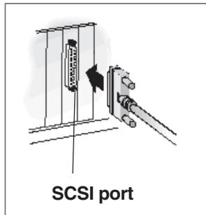
1. With your computer turned off, locate the SCSI port on the back of your computer. This port has 25 small holes in two parallel rows. (For laptop Macintosh computers, such as the Powerbook, the port has 30 small holes in a grid pattern. For Powerbooks, you need to buy an adapter from a commercial supplier.
