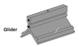
The black anodized aluminum glider has a mass of  $180~g\pm1~g$  and a length of  $129~mm\pm1~mm$ . To increase the mass of the glider simply place the supplied masses on the steel pins protruding from each side of the glider.
