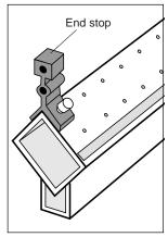
Figure 3 Installing End Stops
