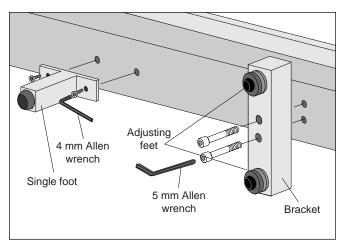
Figure 2 Attaching the Leveling Feet
