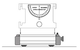
• attached to the side of a PASCO Dynamics Track.
