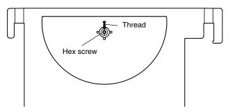
Loosen the hex screw in order to replace the thread. The table shows PASCO part numbers for replacement parts..
