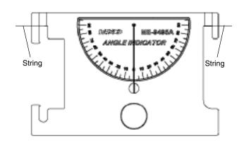
• attached to a PASCO Dynamics Cart, by sliding the device into the slots on the top of the cart.
