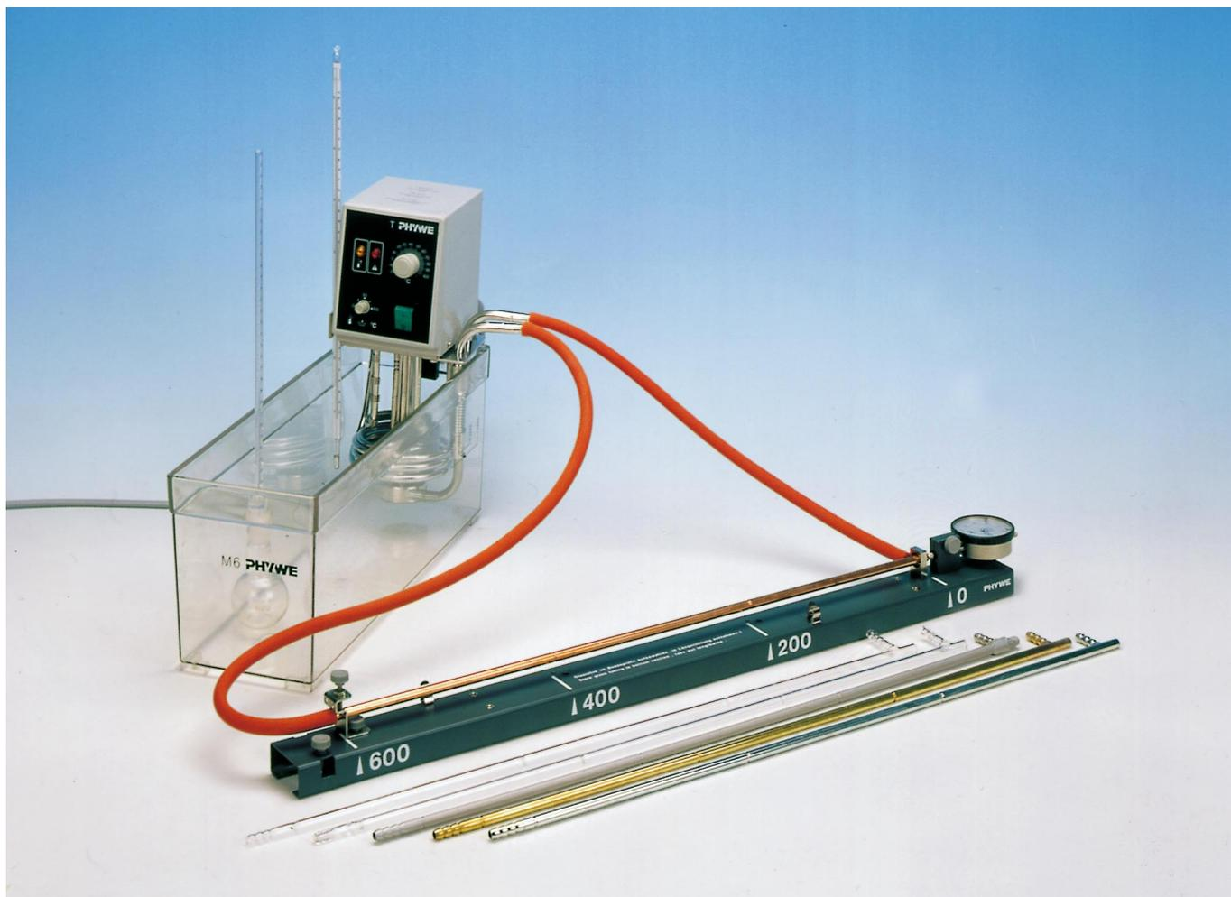
2. The connecting tube to the thermostat is removed and the dilatometer is connected to the water circuit instead. Keep the feed and discharge lines as far away from the dilatometer as possible so that its body will not heat up. Clamp on the measuring tube, set the scale on the dial gauge to "0" and measure the expansion as a function of the temperature.
